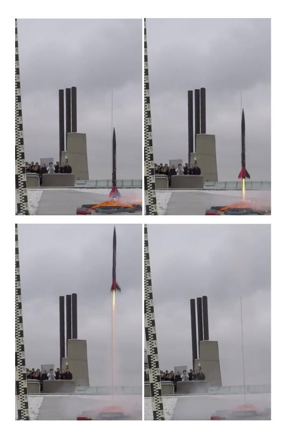
The four video frames on the left show our rocket launch on the roof of the Science Wing. The frames are 75 milliseconds apart. Use these images and the scale on the left to estimate the acceleration of the rocket. Even though this will obviously be only a rough estimate, try to make it as accurate as possible but don't worry about any perspective distortions.
